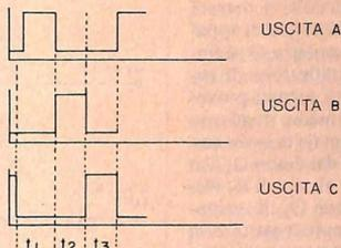
$$t_1 = t_2 = t_3 \text{ Quando } R_1 = R_2 = R_3$$
