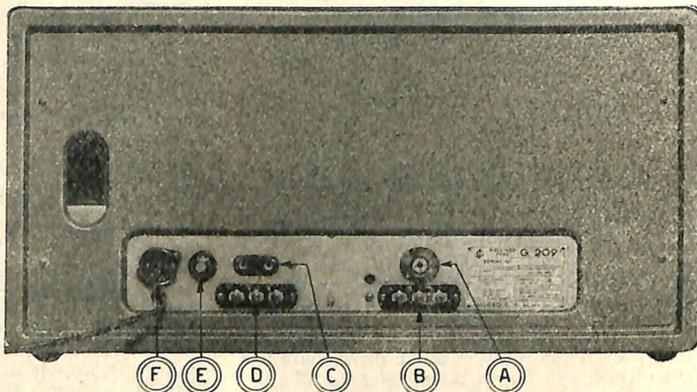
**G 209-R - Rear connections.** A = antenna input for coaxial cable. B = antenna input for balanced line. C = connection for stand-by remote control. D = AF output terminals (impedance: 1-2 = 3,2 ohm; 1-3 = 500 ohm). E = fuse (calibrated 2 A). F = voltage line adjustment switch.
