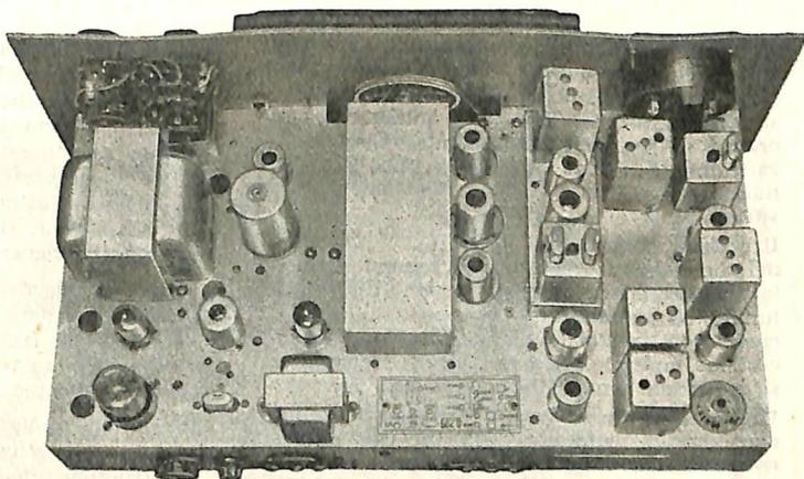
View of chassis mounted with the tubes and X-talls.
