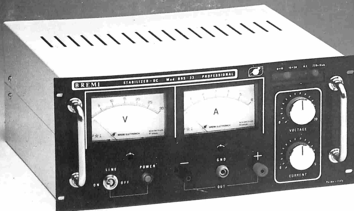
0÷30 VOLT 5 AMPER RIPPLE 200  $\mu$ V
