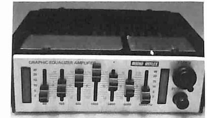
AMPLI-EQUALIZZATORE 25+25 W
