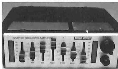
AMPLI-EQUALIZZATORE 25+25 W
