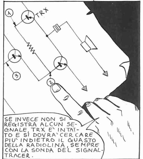
SE INVECE NON SI REGISTRA ALCUN SEGNALE, TRX E' INTATTO E SI DOVRA' CERCARE PIU' INDIETRO IL GUASTO DELLA RADIOLINA, SEMPRE CON LA SONDA DEL SIGNAL-TRACER.
