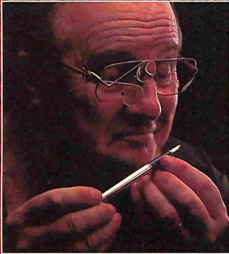
**EXACTING STANDARDS** Key components of every Cross writing instrument are machined to the same degree of accuracy: one one-thousandth of an inch. Craftsman shown inspecting 14 karat gold fountain pen.
