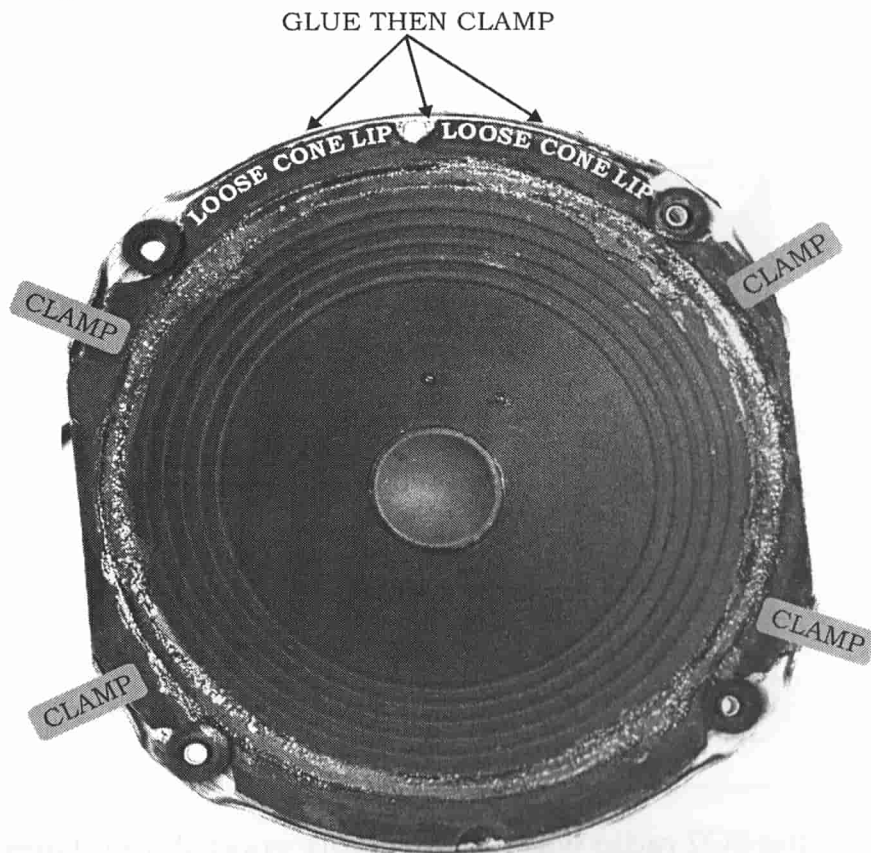
FIGURE 1-11 Speaker with a Loose Cone
