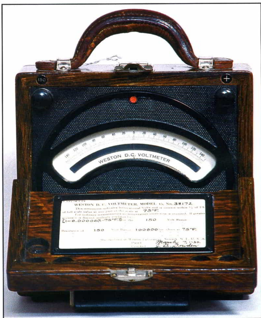
Weston DC voltmeter from 1930 (radio testing equipment).
