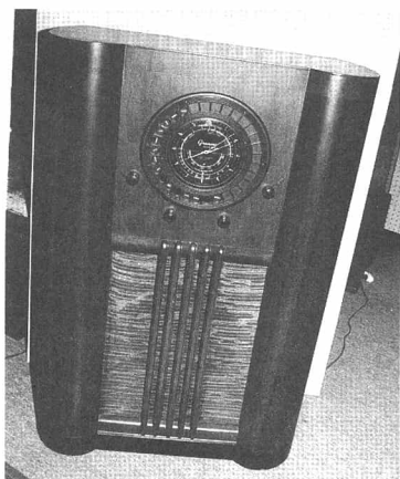
1936 Grunow model 1291, chassis 12B; tele-dial; 12-tube, 4-band (Gene Harris Auctions).
