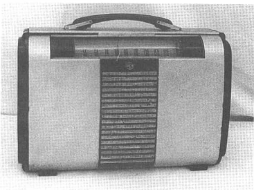
1948 RCA portable model 8 BX 6; operates on both AC and batteries; aluminum and plastic.
