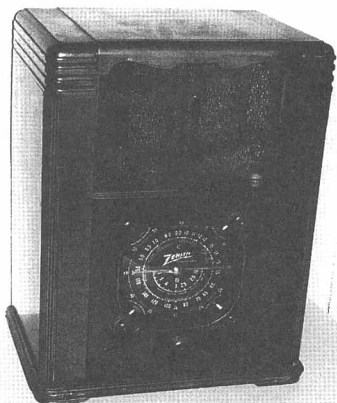
1936 Zenith model 6B129; a 6-volt farm radio.
