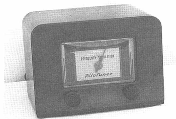
1947 Pilot FM tuner model T-601; played through the phonograph input on a conventional AM radio.
