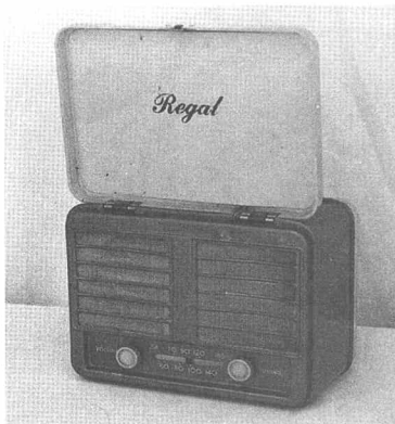
1947 Regal portable model 747; metal case with plastic front and back; flip-up cover; AC/battery operation.
