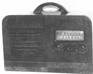
General Motors portable; late 1930s; called a "plug in portable." The middle control switches from AC to battery operation.
