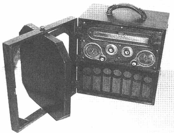
1925 RCA Radiola model 26; portable, loop antenna; battery operated; beautiful wood case with gold-colored dials; original cost $225.00 (Gene Harris Auctions).
