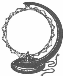
1926 loop antenna made by Eclipse Radio Laboratories; a basketweave antenna could be rotated easily on its pivot.
