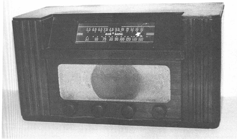
1946 Air King model 4604-D; AM/SW. Reverse painting on dial is flaking off. Watch out for this when buying a set.
