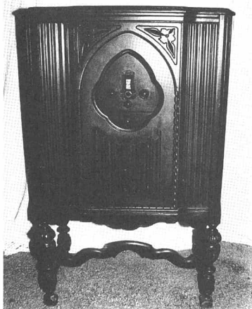
1932 General Motors model 252. A sliding door pulls up to cover the dials when not in use. It’s an unusual radio because the speaker faces out the bottom of the set.
