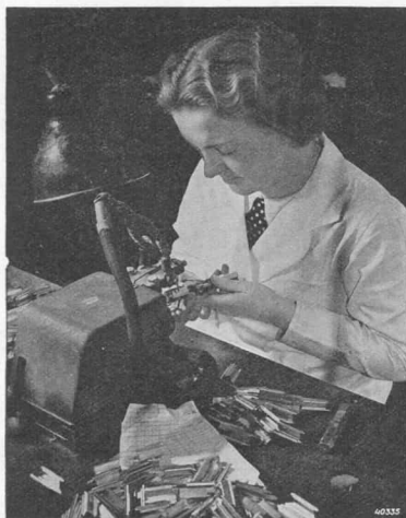
Fig. 69 Spot-welding the supports to anodes and screen plates.
