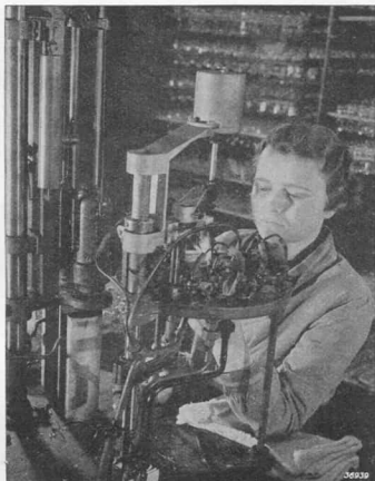
Fig. 74 A thin glass tube is fused to the top of the bulb where the top grid connection is to emerge.
