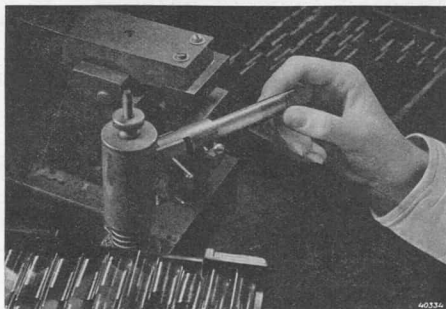
Fig. 67 Checking the dimensions of grids.
