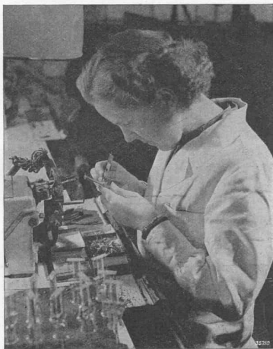
Fig. 80 Mounting the lower mica plate, with cathode and grid already assembled, onto the pinch,
