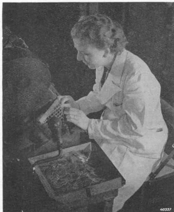
Fig. 72 Punching out mica discs.
