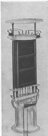
Fig. 115 Electrode system of directly-heated output triode, type AD 1.
