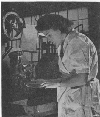
Fig. 73 Machine for cutting and bending the fine wires used for securing the electrodes.
