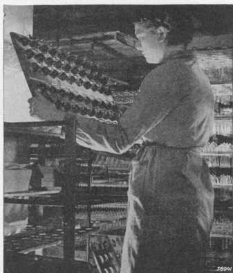
Fig. 75 The bulb is inspected by viewing it against a strongly illuminated frosted glass.
