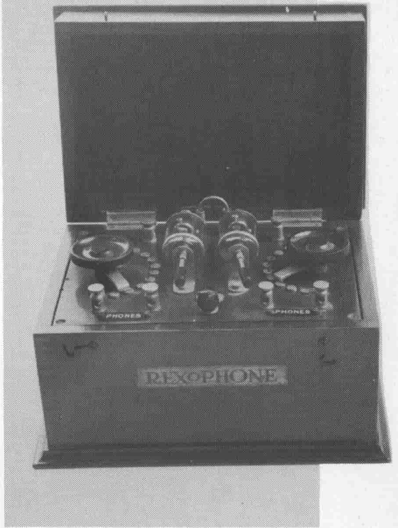
Fig 54 The Rexophone with double crystal. GPO No.792. Made by Morch Bros. Ltd.
