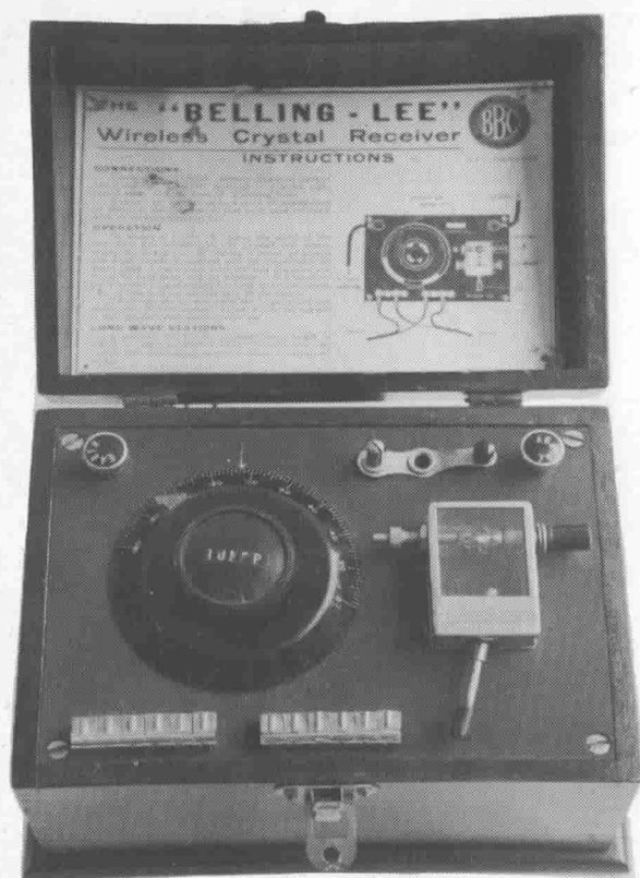
Fig 39 Belling Lee crystal set. GPO Number 4553
