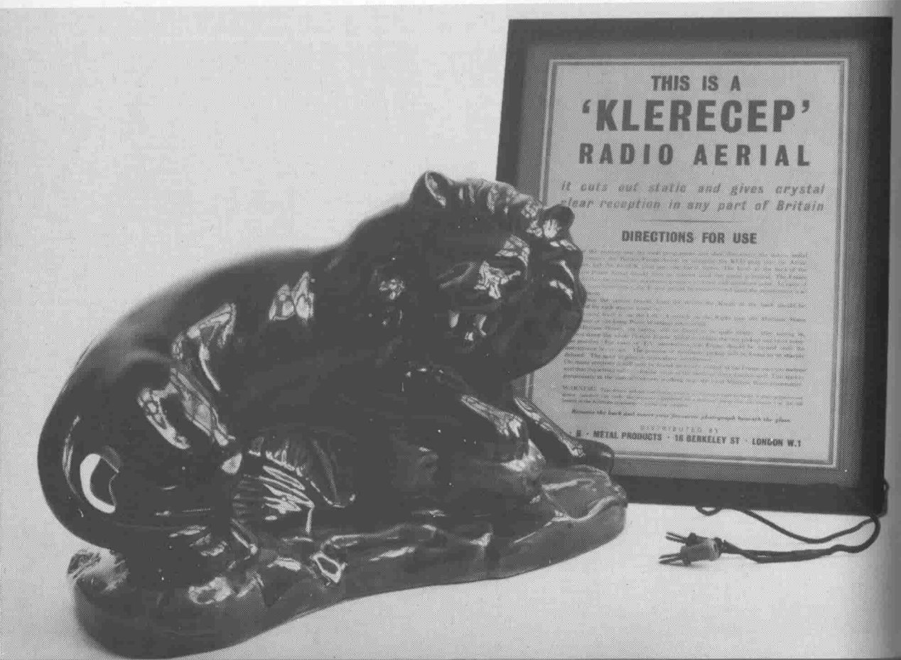
Fig 140 The lion disguises a frame aerial. The picture frame also contains a frame aerial.
