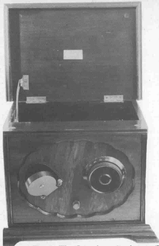
Fig 85 The Gecophone 2 valve set (BC 2720). Detector, L.F. with variable aerial reactance unit. Transformer coupled.
