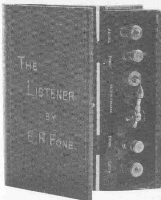
Fig 135 & Fig 136 A novelty crystal set made in about 1926 by Kenmac Radio Ltd. This crystal set has tapped inductance tuning. It came in green or red rexine or tortoiseshell finish.
