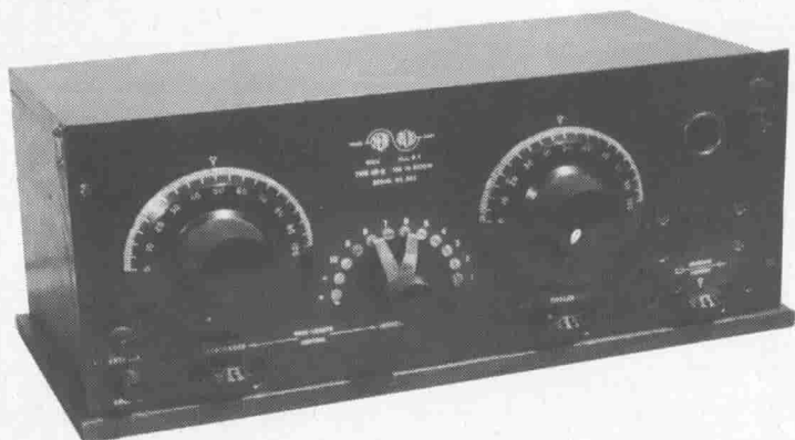
Fig 108 A one valve regenerative receiver, model CR5 made by A.H. Grebe & Co. 1921.
