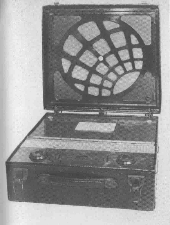
Fig 160 The McMichael 'Duplex Four' TRF portable in leather case. This was one of the higher quality suitcase portables so popular for motoring picnics. 1932.
