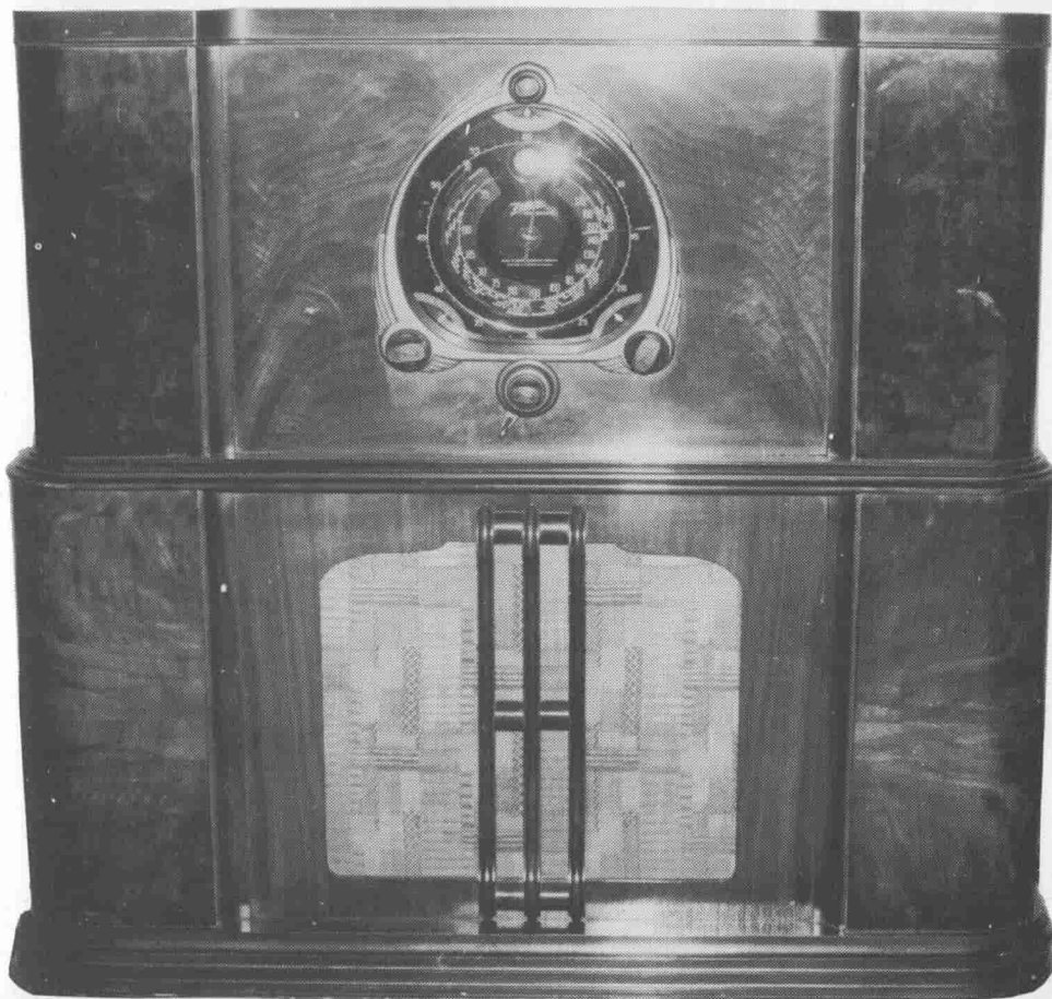
Fig 167 Zenith Radio Corp. Model 9S264. Nine valve AC mains superhet. USA 1938.
