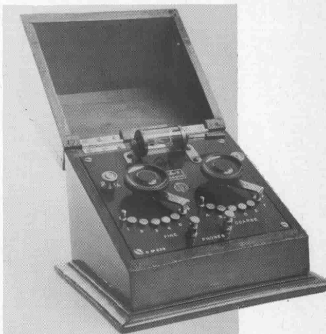
Fig 48 (above) Gecophone No.1. Mahogany box. This set also came in a version with a glass enclosed crystal. GPO No.102
