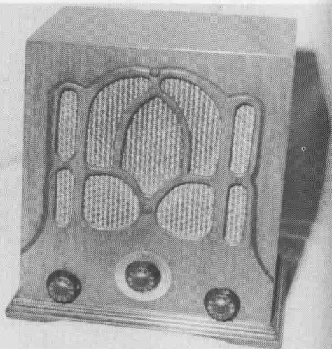
Fig 164 Zenith Radio Corp Model 805. Five valve AC mains superhet (left). Trot Mfg Co. Model 44. Four valve AC mains TRF (right) USA 1934.
