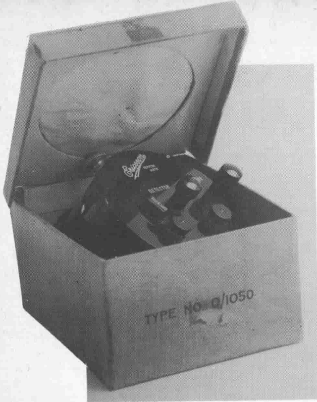
Fig 45 Ericsson Crystal set, type 0/1050. Miniature, turned polished ebonite. Cardboard container is 2" square and 1½" deep. GPO No.5228
