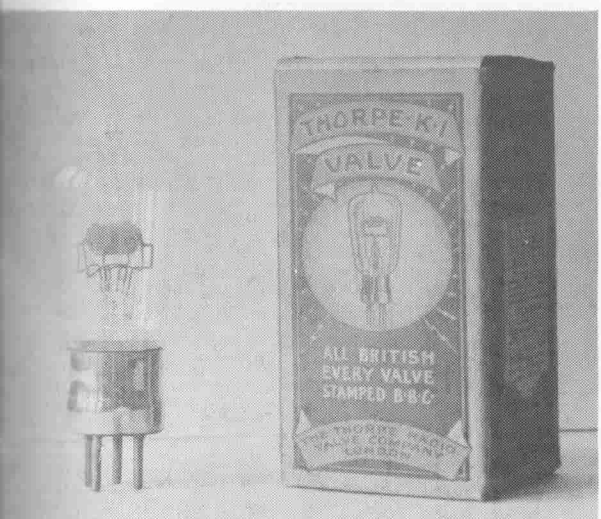
Fig 127 Introduced in 1924, the Thorpe K1 has the unusual feature of a helically wound anode.
