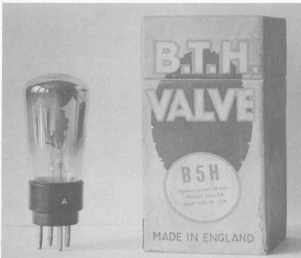
Fig 130 The BTH B5H for high frequency amplification first appeared in 1923.
