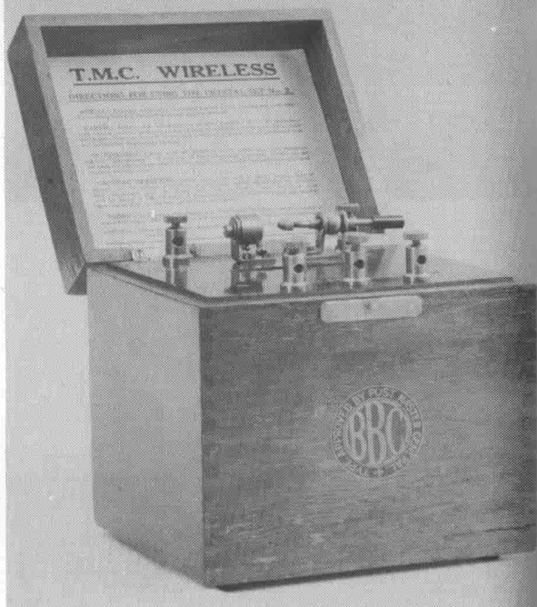
Fig 57 The T.M.C. crystal set made by the Telephone Manufacturing Co. GPO No.183.
