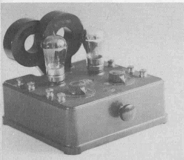
Fig 80 Burndept's Duplex VA in black composition moulded case.
