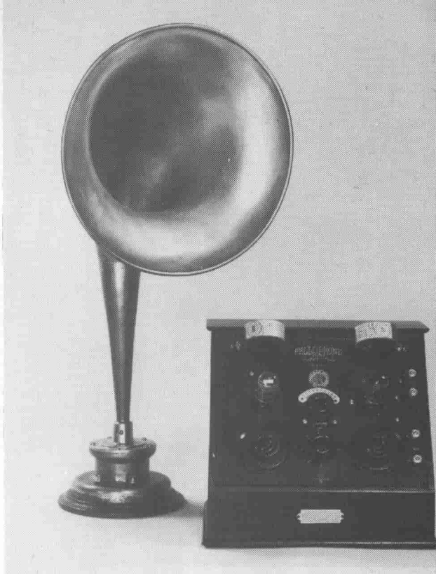
Fig 65 Fellowphone Super Two manufactured by the Fellows Magneto Co., Ltd.) H.F. and detector. GPO No.226. The speaker is by TMC.
