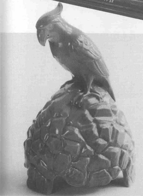
Fig 100 A heavily disguised speaker made by Andia (Doulton & Company) with an Amplion drive unit. Green glazed pottery.
