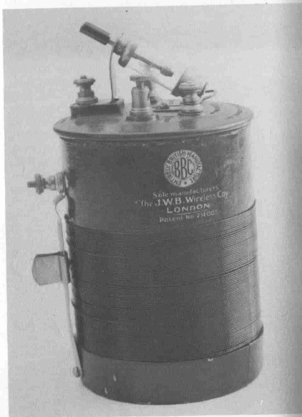
Fig 70 Tubular crystal set made by J.W.B. Wireless Company. This company was later called Brownie Wireless Co. and the sets were called 'Brownie'. Note the later version of the BBC stamp. Earlier versions of this model bore the GPO No.4155.
