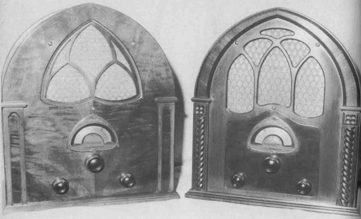
Fig 163 Atwater Kent Mfg Co. Model 82. Seven valve C mains superhet (right) and Model 84. six valve AC mains superhet. USA 1932.
