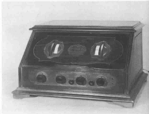
Fig 120 (below) RCA Model Radiola 20 five valve TRF receiver. 1925.
