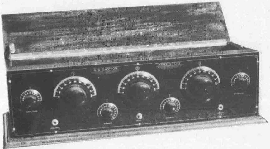
Fig 122 A.C. Dayton Co., Model XL5 five valve TRF receiver. 1925.
