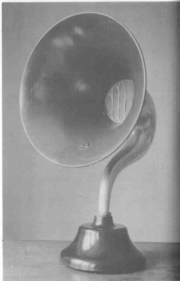
Fig 98 B.T.H. C2 speaker first introduced in 1924. It gradually evolved into this streamlined bakelite and aluminium version and was still available in the late 1920s. Over a million of them were made.
