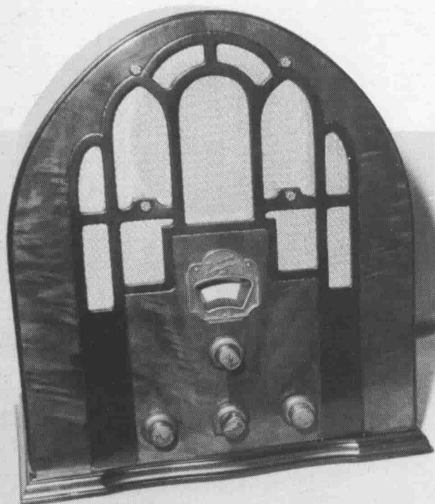
Fig 164 Zenith Radio Corp Model 805. Five valve AC mains superhet (left). Trot Mfg Co. Model 44. Four valve AC mains TRF (right) USA 1934.
