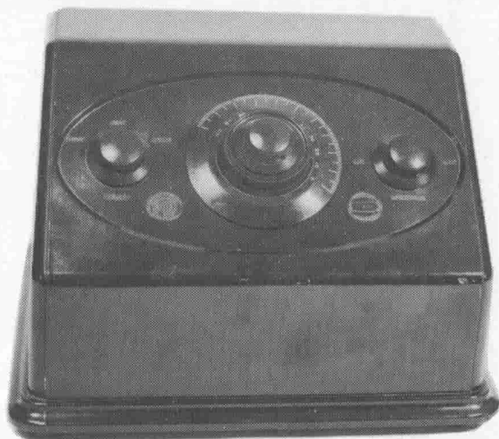
Fig 91 Pye 232 in moulded bakelite case. The use of bakelite was cautious at this stage but soon began to have an impact on cabinet design. This is a 2 valve battery operated set. c 1928
