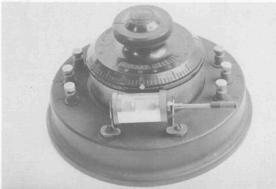
Fig 41 The Cosmos crystal receiver in moulded case 'Type Approved' but GPO number not known.
