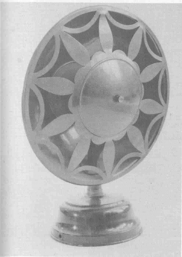
Fig 104 The Nesper reflex bowl speaker. The whole structure is made of lightweight metal and resembles the cone speakers in appearance and dimensions.
