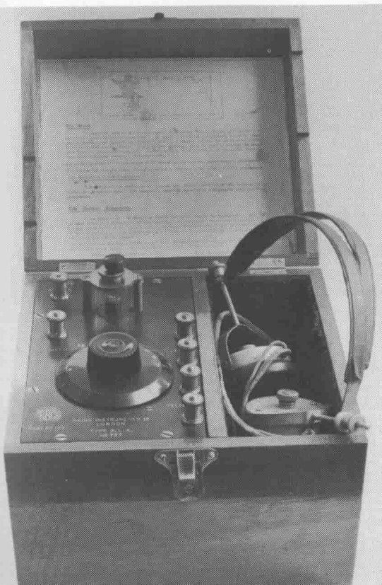
Fig 53 The Revophone crystal set. Mahogany box. GPO No.669. Made by Cable Accessories Co.
