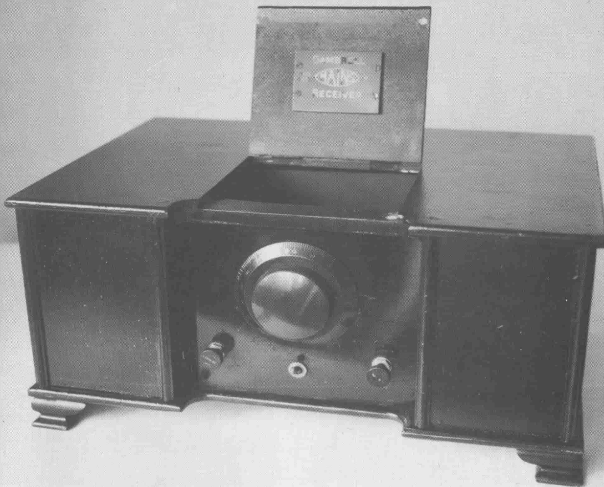
Fig 88 Gambrell Model C2DC mains operated set. Made in about 1927. This was one of the first British mains sets commercially available.
