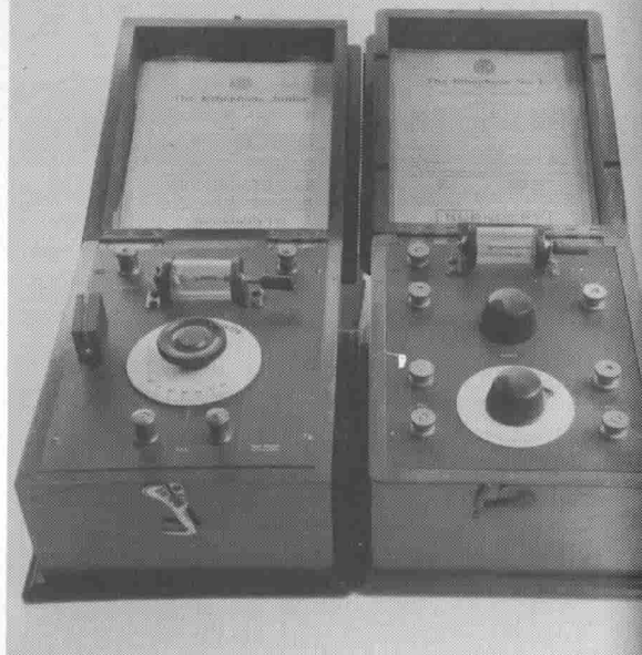
Fig 40 Two crystal sets by Burndep, the 'Junior' (GPO No.113) and the Ethophone No.1, Mk III (This set appeared after the GPO No. period)
