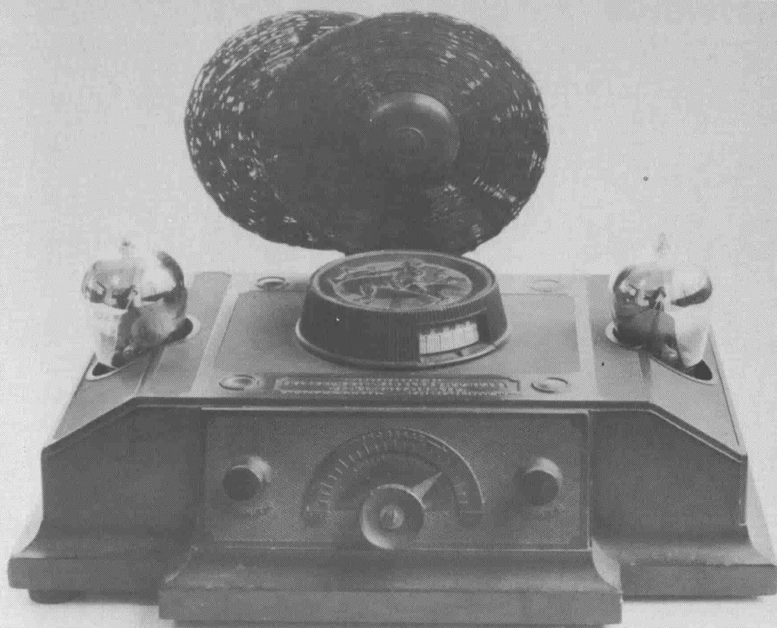
Fig 79 Brownie 2-valve set. Made by Brownie Wireless Co. who specialised in moulded cases.
