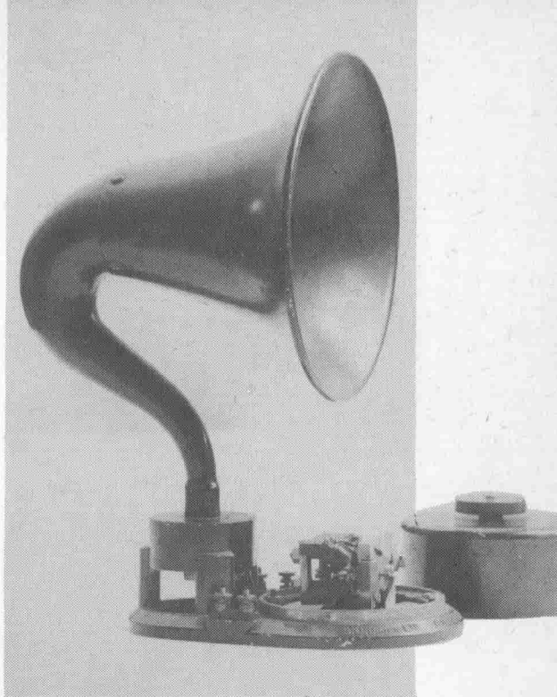
Fig 95 The Crystavox speaker by S.G. Brown. This speaker has a built-in microphone amplifier — a speciality of this company. The knob on the amplifier cover has a magnet attached to it which finely controls the balance of the amplifier armature.
