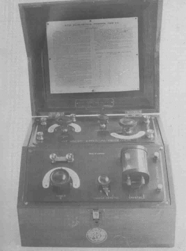
Fig 64 BTH (British Thomson-Houston Co. Ltd., Rugby) H.F. valve, crystal detector receiver. GPO No.0373
