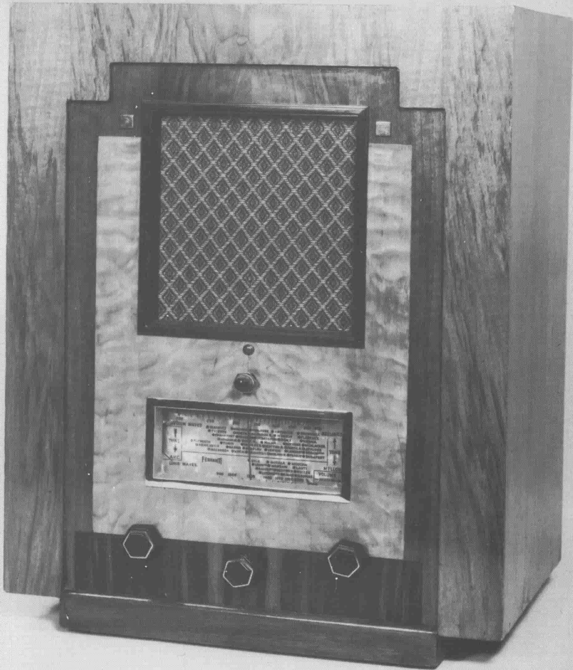
Fig 158 The Ferranti 'New Arcadia'. Four valve AC mains superhet. Veneered wood case. 1934.
